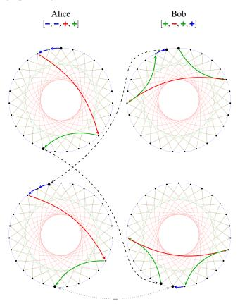
Figure 9: Key exchange on a regular isogeny graph.
